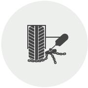
The Onspot Automatic Tire Chain System is an uncomplicated yet very reliable solution for increasing traction. It's a chain wheel attached to a rotatable arm that in turn is permanently mounted on the vehicle.
