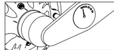
Caution! Do not bend the magnet with the spring during installation and removal.
