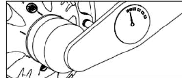
Caution! Do not bend the magnet with the spring during installation and removal.
